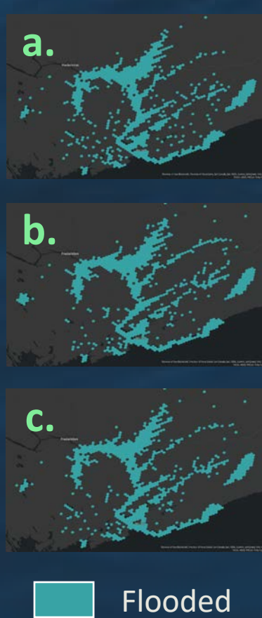
Fig. 4 Prediction of the flood extent in ISEA3H DGGs at levels a. 19, b. 21, and c. 23.
