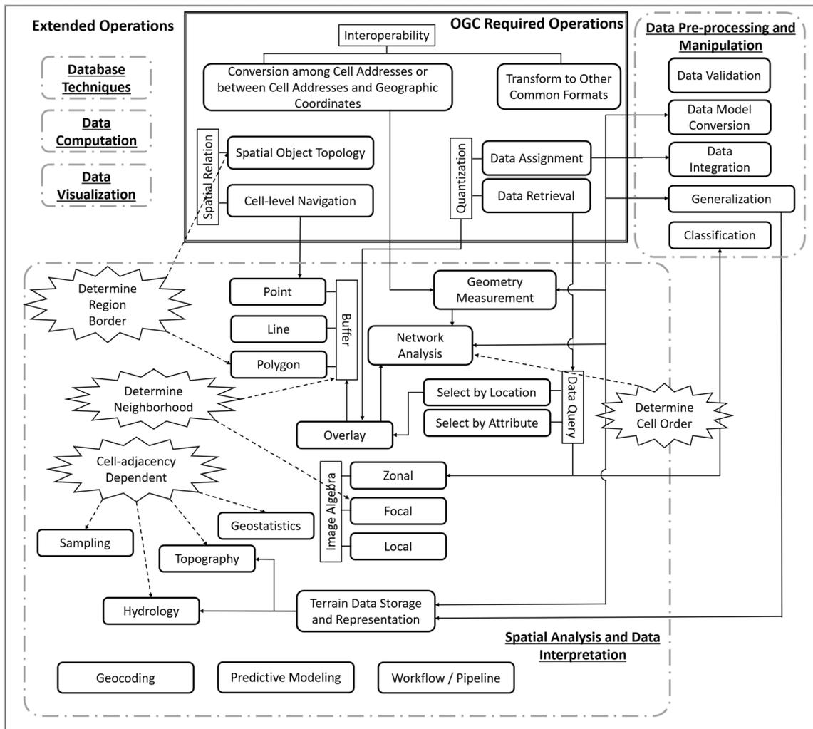
**Fig. 3** The OGC required operations and the extended DGGS operations discussed in this paper. Arrows mean that the development of the prior can facilitate the development of the latter operation
