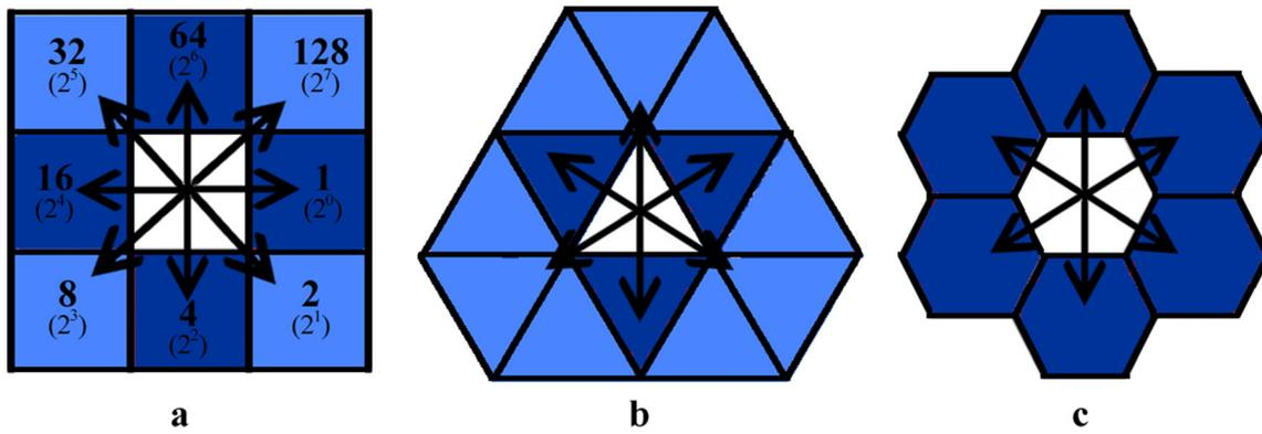
Fig. 4 Flow directions on a square, b triangular, and c hexagonal grids
