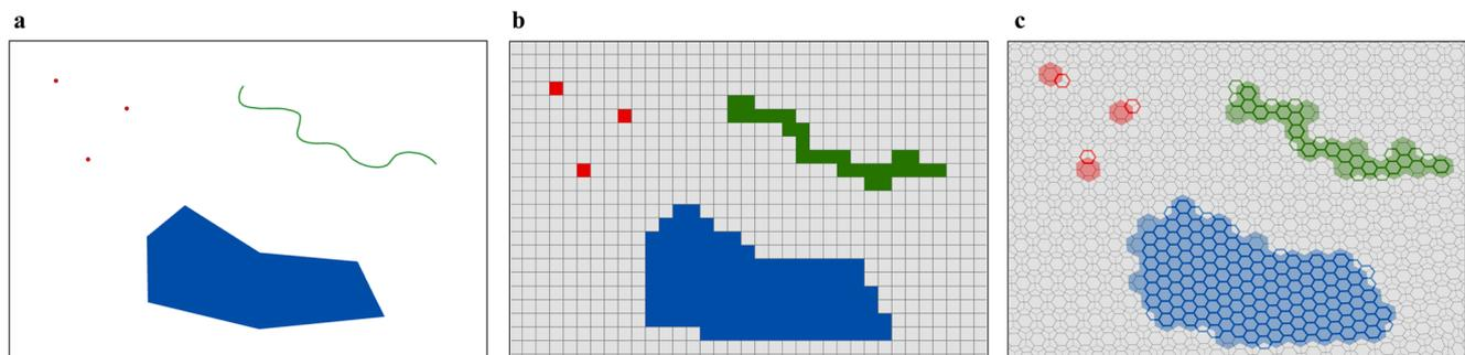
**Fig. 1** Modeling spatial objects by **a** the vector model, **b** the raster model, and **c** the hexagonal DGGS model at two different resolution levels: solid cells and hollow cells represent the modeling at the coarse and fine resolutions, respectively
