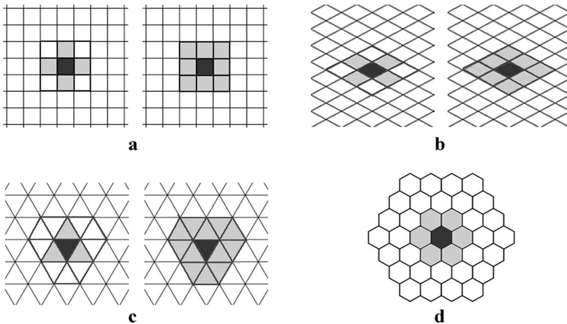
Fig. 5 a Rook’s case (left) and Queen’s case (right) contiguity on square grids, b pseudo Rook’s case (left) and Queen’s case (right) on diamond grids, c pseudo Rook’s case (left) and Queen’s case (right) on triangular grids, and d adjacent contiguity on hexagonal grids
